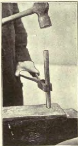
FIG. 12. SQUARING AN END, ALSO UPSETTING.
