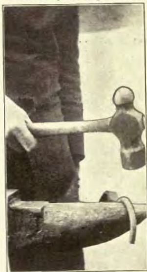
FIG. 13. BENDING OVER THE HORN OF THE ANVIL.
