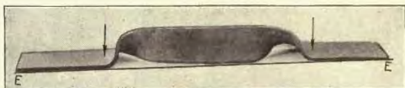
FIG. 34. CENTER HAMMERED TO ONE SIDE; ENDS HAMMERED DOWN AT ARROWS.
