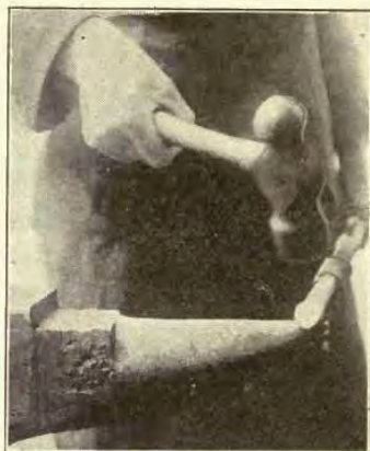
FIG. 43. BENDING POINT OF SCARF.
